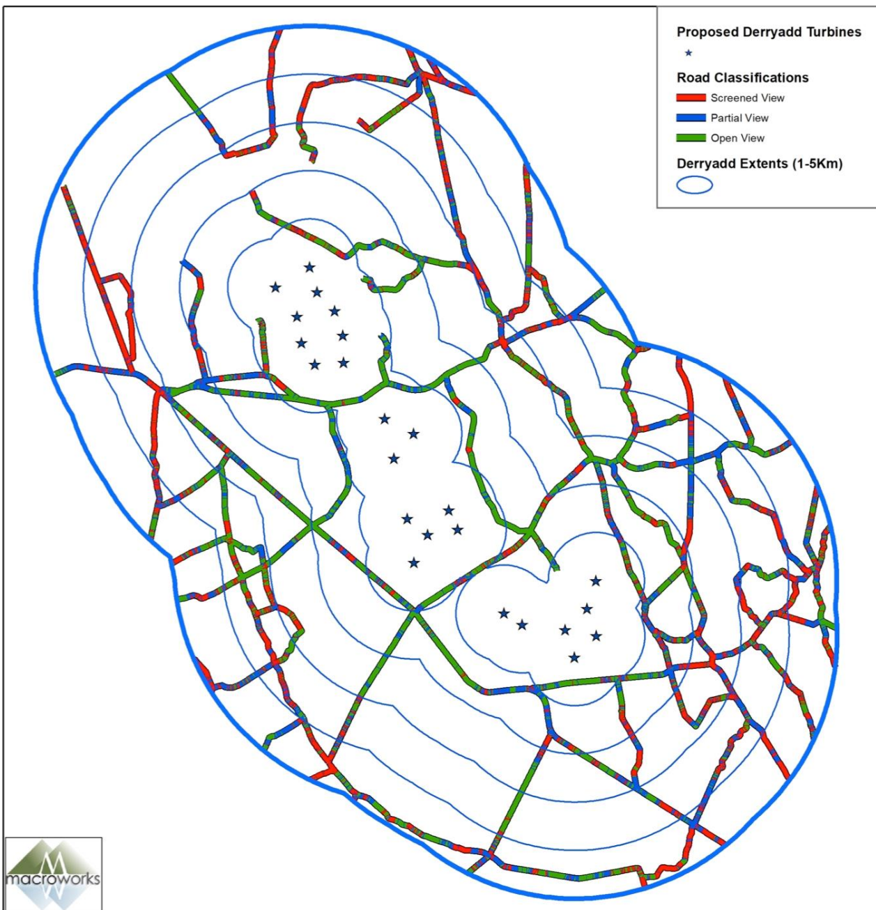
Figure 9.10: Map of Route Screening Analysis for roads within 5km of turbines (See Appendix 9.1 for larger scale map)
